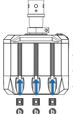
Insert the T-nuts into the T-slots found on the underside of the wheel base for hard-mounting from the bottom.
