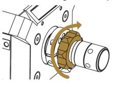
Simplified Quick Release: carefully push the steering wheel onto the shaft. Use the M6x20 screw from the Podium Wheel Base accessories for tightening the clamping ring.
