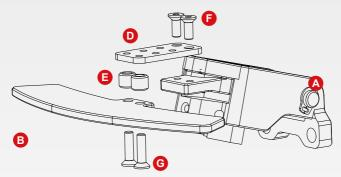
42 Setup for steering wheels with a diameter smaller than 28 cm (Formula):
